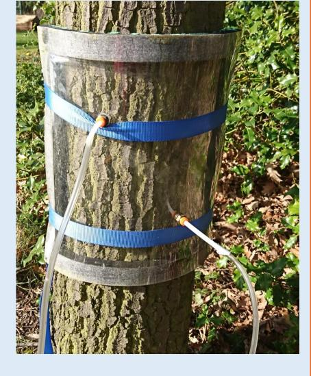
The greenhouse gas analyser will measure the concentration of CH<sub>4</sub> in the chamber.
