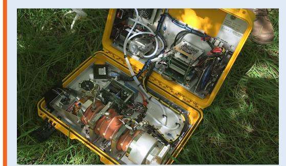
This can be used to determine the amount of CH<sub>4</sub> emitted or taken in by a tree over time.
